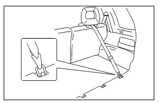
Your vehicle's top strap anchors for the rear seating positions are located on the floor of the rear cargo area, along the outside edge. If your vehicle is equipped with a luggage compartment cover, remove it before using the top strap. When routing the top strap at an outboard seating position, pass it between the head restraint and the rear seatback.
